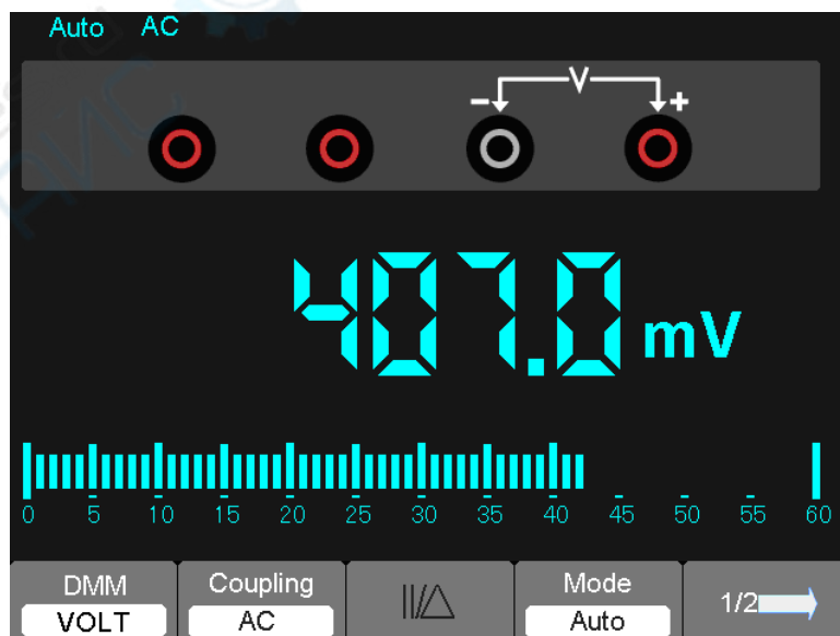
Figure 7-7 AC voltage Measurement
